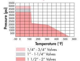
**Note:** Carbon Steel valves are limited to -20°F.
